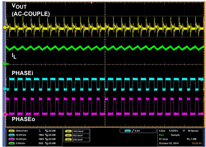
FIGURE 7. OUTPUT RIPPLE AT 1A LOAD ( V_{IN} = 8V )
