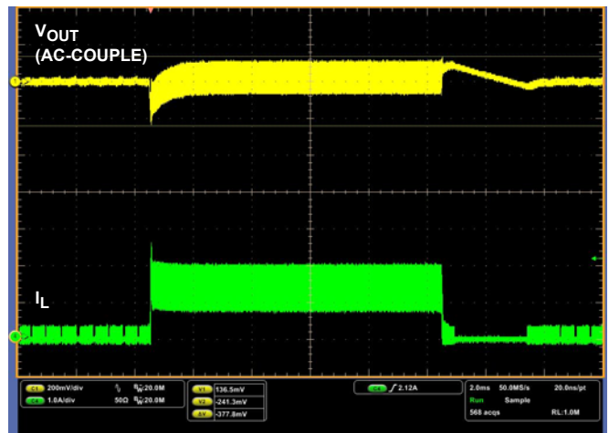
FIGURE 11. LOAD TRANSIENT RESPONSE 0A->1A, V_{IN} = 36V
