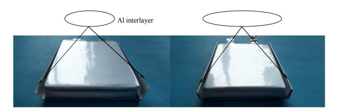
Fig.2. Single folding edge schematic of PL cells schematic of PL cells
