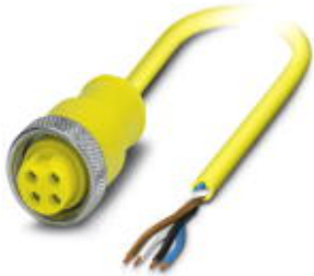
Sensor/Actuator cable, 4-position, PVC, Yellow RAL 1021, Free cable end, on Socket straight 7/8"-16UNF, A-coded, Cable length: 4 m
