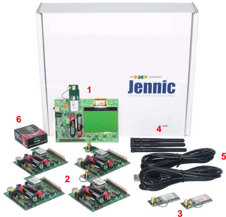
Figure 1: JN5148-EK010 Evaluation Kit Components
