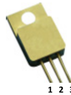
TO – 257 (Isolated Base-plate Hermetic Package)
