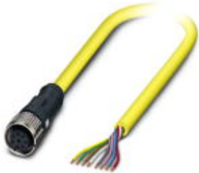
Sensor/Actuator cable, 8-position, PVC, yellow, Free cable end, on Socket straight M12-SPEEDCON, A-coded, Cable length: 2 m
