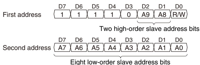
Figure 14.4.4.1 10-bit Address Configuration
