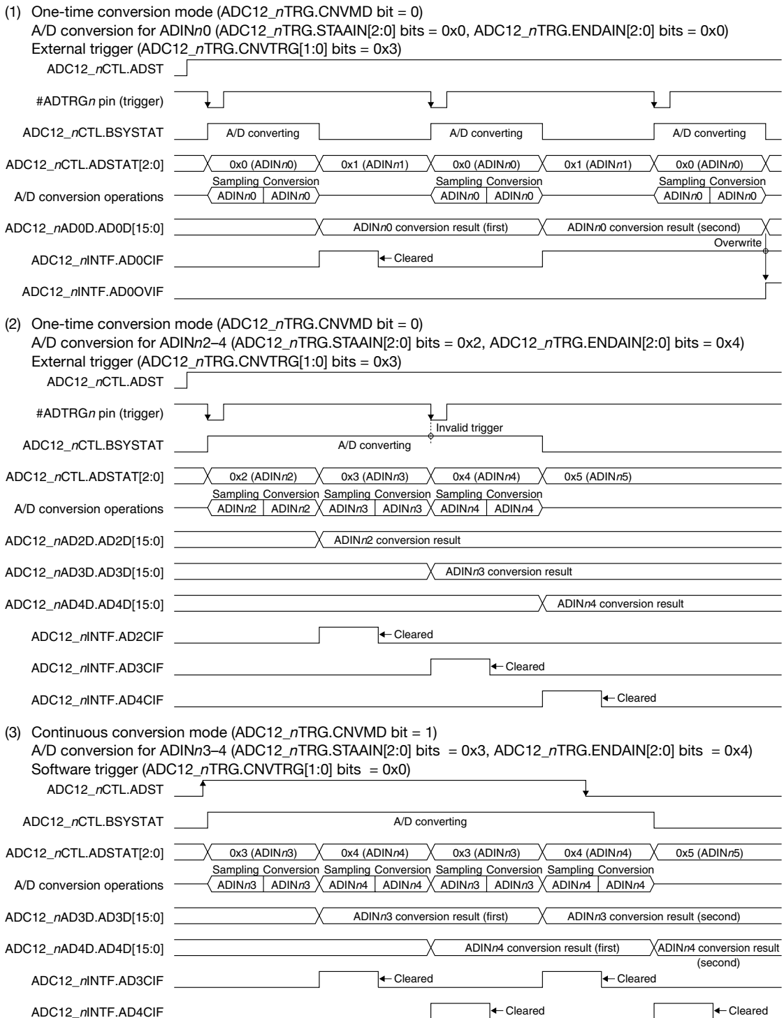
Figure 20.4.4.1 A/D Conversion Operations
