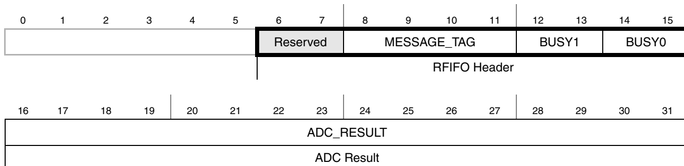
Figure 18-32. Result Message Format for External Device Operation
