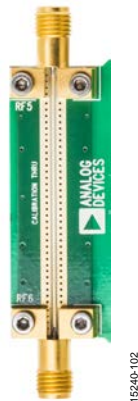
Figure 2. EVAL-ADGM1004EBZ Calibration Transmission Line Used for PCB Insertion Loss and Phase Offset Correction
