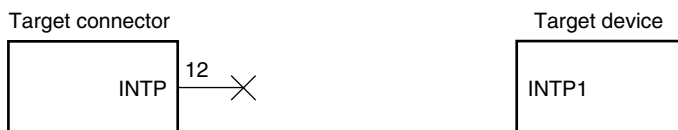
Figure 17-3. Circuit Connection for the Case Where QB-MINI2 Is Used Only for Programming
