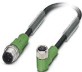
Sensor/actuator cable, 3-position, PUR halogen-free, black-gray RAL 7021, Plug straight M12, A-coded, on Socket angled M8, cable length: 1.5 m
