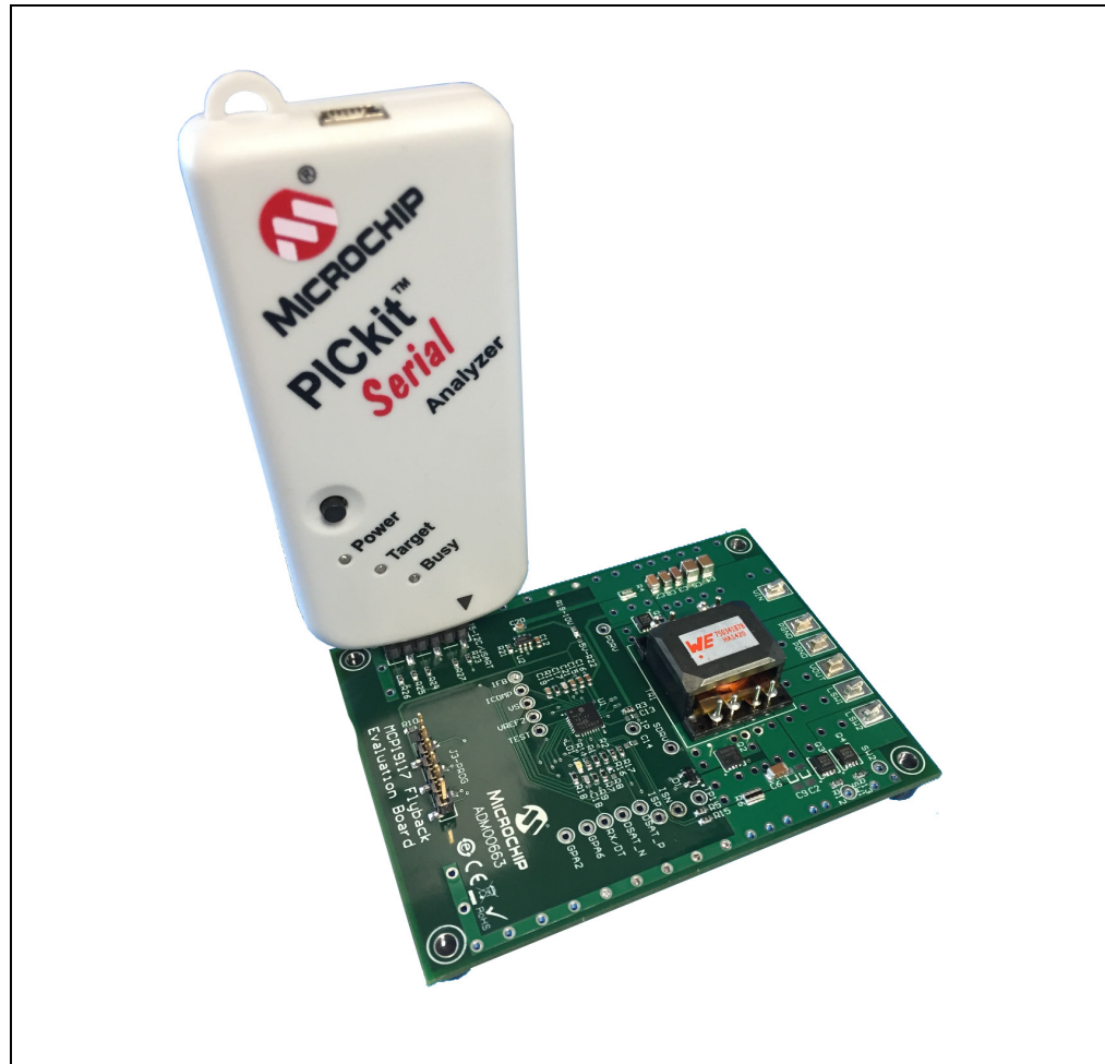
FIGURE 3-1: PICKit Serial Analyzer Connection to the Board.
