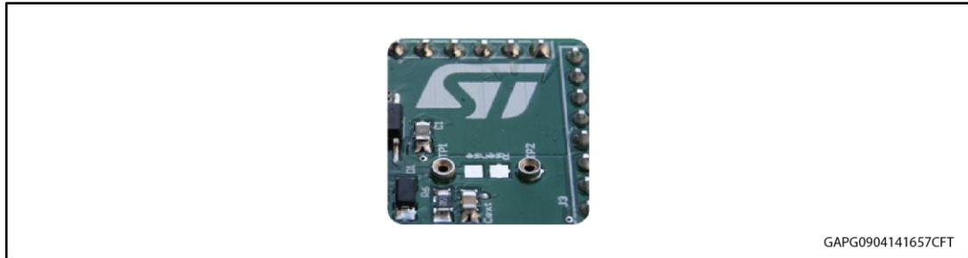
Figure 4: Mounting through-hole sense resistor
