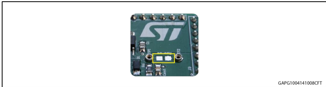
Figure 5: Pads for soldering SMD resistor
