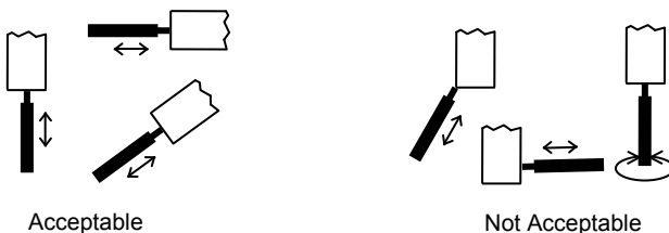
Figure 1 – Correct and Incorrect Angles of Measurement
