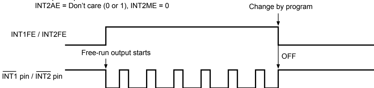
Figure 26 Output Timing of User-set Frequency
