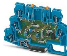
Double wire (loop), intrinsically safe, e.g., for 4 ... 20 mA current loops
