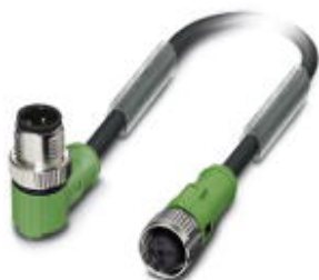
Sensor/actuator cable, 3-position, Variable cable type, Plug angled M12 SPEEDCON, A-coded, on Socket straight M12 SPEEDCON, A-coded, PIN 2+4 bridged, cable length: Free input (0.2 ... 40.0 m)
