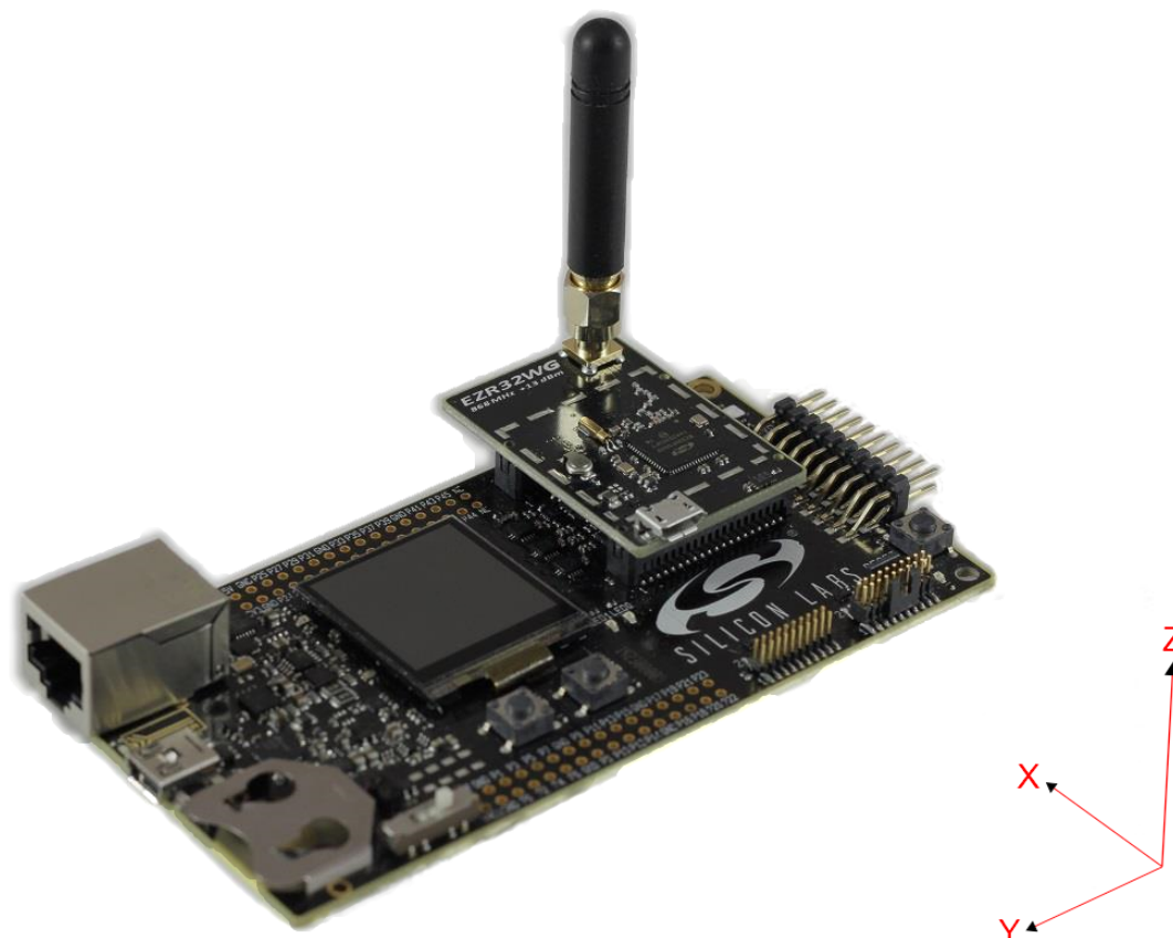
Figure 6.2. DUT: BRD4503B (Rev. A00) Radio Board with Wireless Starter Kit Mainboard
