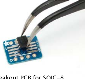
SMT Breakout PCB for SOIC-8, ( /products/1212 )
