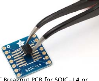
SMT Breakout PCB for SOIC-14 or ( /products/1210 )
