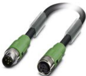
Sensor/Actuator cable, 5-position, PUR, Black-gray RAL 7021, Plug straight M12-SPEEDCON, A-coded, on Socket straight M12-SPEEDCON, A-coded, Cable length: 3 m
