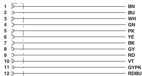
Contact assignment of the M12 socket
