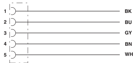
Contact assignment of 7/8" socket
