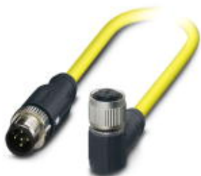
Sensor/Actuator cable, 5-position, PVC, yellow, shielded, Plug straight M12 SPEEDCON, A-coded, on Socket angled M12 SPEEDCON, A-coded, Cable length: 0.5 m
