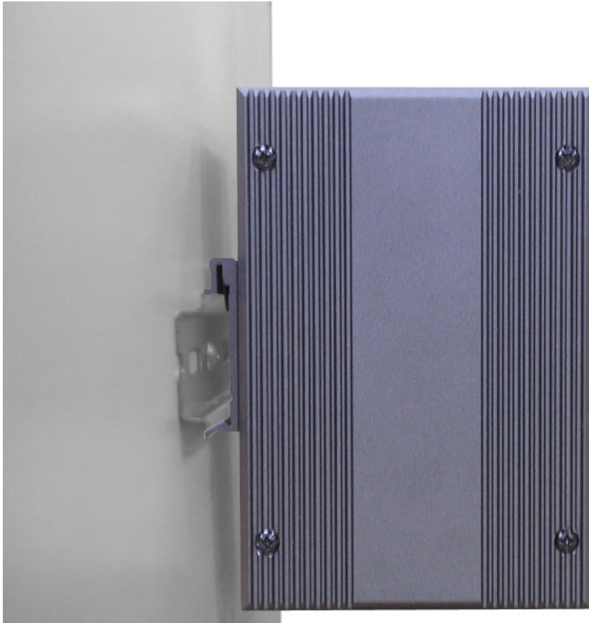
Figure 2.7: Installation to DIN-rail Step 2
