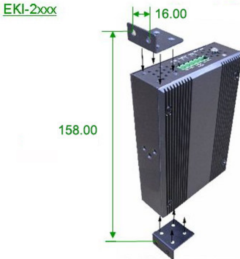
Figure 2.5: Combine the Metal Mounting Kit (units: mm)
