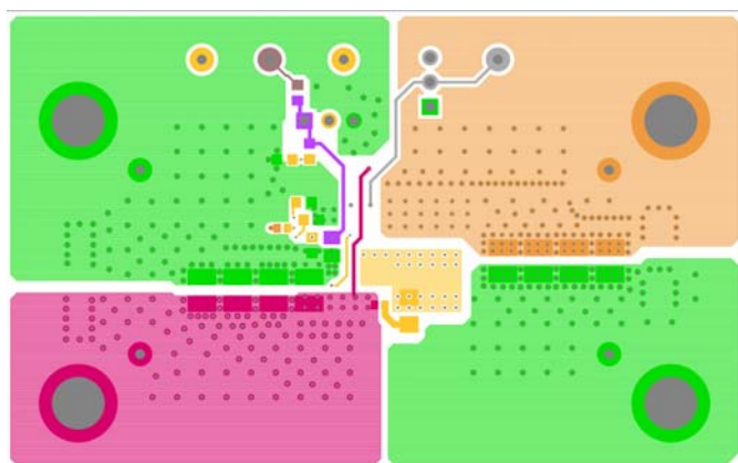
Figure 9. Bottom Layer Solder Side
