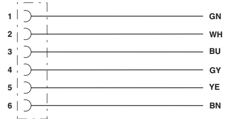
Contact assignment of 7/8" socket
