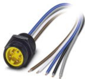
Flush-type connector, 5-position, Plug, straight, 7/8"-16UNF, on free cable end, Front mounting, with 1/2 inch-14 NPT mounting thread, Individual wires, cable length: 1 m
