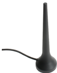
Figure 15. Mike 1A GSM antenna
